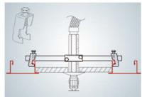
Modular grid and panel ceiling systems with C, Z or U-shaped profile rails (recommended minimum width for mounting on C or U-shaped profile rails 100 mm)
