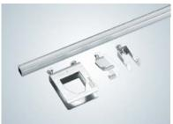
The sprinkler bracket type 4 is especially suited for floor-ceiling systems. The square pipe (length 2000 mm) is attached directly to the C, Z or U-shaped profile rail running near the wall using type 4 mounting clips.
