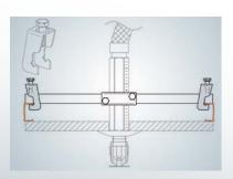
Grid ceiling system with Z-shaped profile rails
