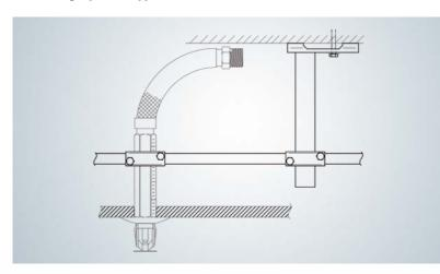
The sprinkler hose is attached using this bracket, regardless of the construction and geometry of the suspended intermediate ceiling. The base supporting beam is anchored directly on the concrete ceiling. The sprinkler can be positioned as required in a radius of 600 mm around the mounting position of the base supporting beam. The side lateral offset can be implemented using a square pipe, which is securely screwed onto the pipe of the base supporting beam using a sprinkler clamp.
