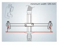
Modular grid ceiling – installation between two U-shaped profile rails
