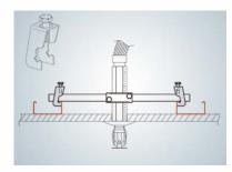
Plasterboard ceiling with mounting clips
